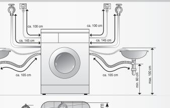
The drain hose should not be placed higher than 100 cm above the floor.
