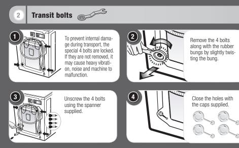
) Keep the 4 bolts and the spanner for the future use. Refit transit bolts before transporting the appliance.
