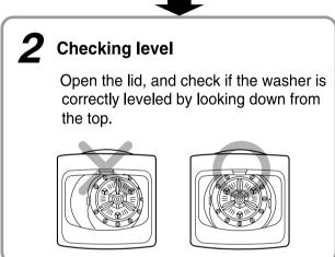
Improper installation of the washer may cause noise and malfunctioning.
