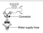
4. Fixing the connector of connector and water supply hose
