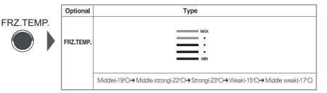
How to adjust the temperature in the refrigerator compartment
