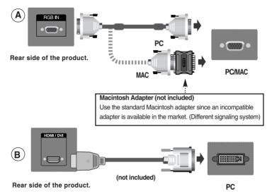
\* User must use shielded signal interface cables (D-sub 15 pin cable, DVI cable) with ferrite cores to maintain standard compliance for the product.
