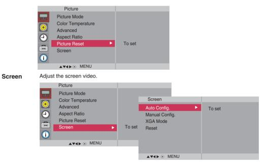
Auto Config. (RGB PC input only) : This button is for the automatic adjustment of the screen position, clock and phase. This function is available for analog signals only. Manual Config. : If the picture isn't clear after auto adjustment and characters are still trembling, adjust the picture phase manually.
