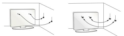
Insert the eye-bolts (or TV brackets and bolts) to tighten the product to the wall as shown in the picture.
