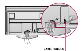
Install the CABLE MANAGEMENT CLIP as shown.
