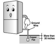
The incorrect grounding may cause breakdown and electric shock.
