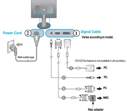
For Apple Macintosh use, a separate plug adapter is needed to change the 15 pin high density (3 row) D-sub VGA connector on the supplied cable to a 15 pin 2 row connector.
