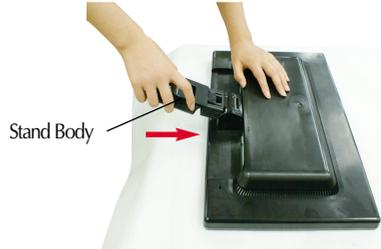
3. Assemble the Stand Base into the Stand Body in the correct direction.
