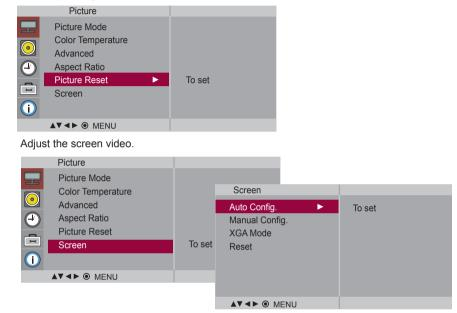
Auto Config. (RGB PC input only): This button is for the automatic adjustment of the screen position, clock and phase. This function is available for analog signals only. Manual Config. : If the picture isn't clear after auto adjustment and characters are still trembling, adjust the picture phase manually.
