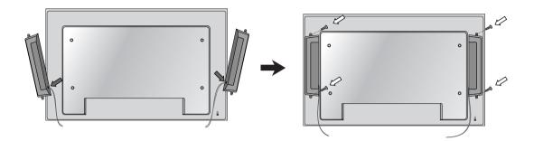
After installing your speakers, use holders and cable ties to organize the speaker cables.
