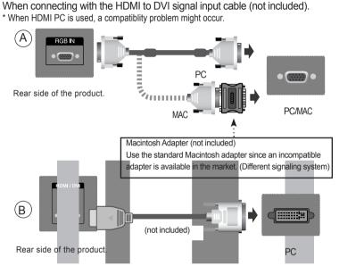
\* User must use shielded signal interface cables (D-sub 15 pin cable, DVI cable) with ferrite cores to maintain standard compliance for the product.
