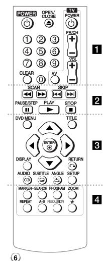
POWER (<sup>(</sup>): Switches the unit ON or OFF. OPEN/CLOSE (**▲**): Opens and closes the disc tray. Numerical buttons: Selects numbered items in a menu.
