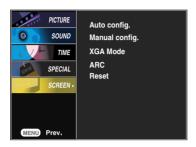
Auto-config. (RGB PC input only) This button is for the automatic adjustment of the screen position, clock and phase. This function is suitable for analogue signal input only.
