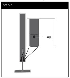
**4.** Connect the speaker wire to the terminal on the speaker.
