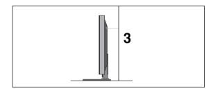
3 Use a sturdy rope to tie the product for alignment. It is safer to tie the rope so it becomes horizontal between the wall and the product.
