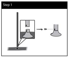
**2.** Insert a speaker wire from the bottom of the base.
