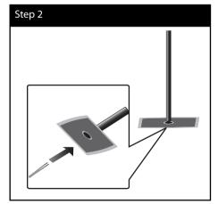
**3.** Draw the speaker wire through the inside of the pole and also through the hole on the bottom of the speaker.
