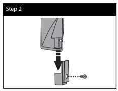
**3.** Hang the speaker bracket onto the wall bracket.
