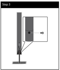
**4.** Connect the speaker wire to the terminal on the speaker.
