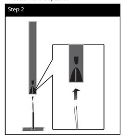
**3.** Attach the speaker to the pole, then secure the connection with a supplied screw.
