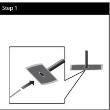
2. Draw the speaker wire through the inside of the pole and also through the hole on the bottom of the speaker.
