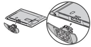
Fix the 4 bolts securely using the holes in the back of the TV.
