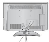
Install the CABLE MANAGEMENT CLIP as shown.
