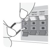
Connect the red end of each wire to the terminals marked +(plus) and the black end to the terminals marked - (minus).
