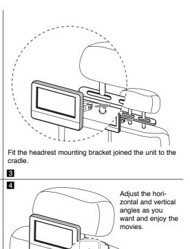
**Note:** When you adjust angles, loose the adjusting screws. Adjusting by force can lead the damage to the inside of your headrest mounting bracket.
