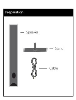
Attach the speaker to the stand, then secure the connection with a supplied screw. Draw the speaker wire through the inside of the stand and also through the hole on the bottom of the speaker.
