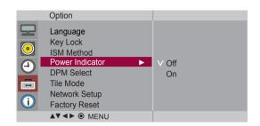
**Power Indicator** Use this function to set the power indicator on the front side of the product to On or Off. If you set Off, i will go Off. If you set On at any time, the power indicator will automatically be turned on.
