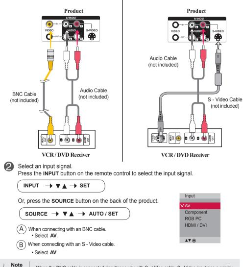
. When the BNC cable is connected simultaneously with S - Video cable, S - Video input has a priority.
