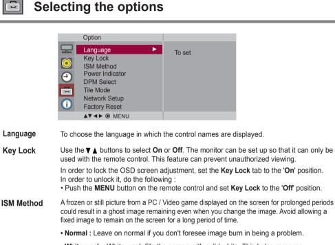
• White wash : White wash fills the screen with solid white. This helps removes permanent images burned into the screen. A permanent image may be impossible to clear entirely with white wash.
