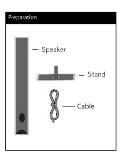
Attach the speaker to the stand, then secure the connection with a supplied screw. Draw the speaker wire through the inside of the stand and also through the hole on the bottom of the speaker.
