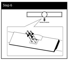
**7.** Hang the main unit onto the brackets, as shown below.
