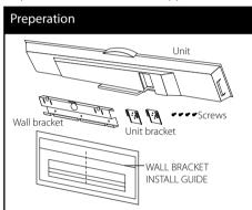
2. When you mount it on a wall (concrete), use the wall plugs (Not supplied). You should drill some holes. A guide sheet (WALL BRACKET INSTALL GUIDE) is supplied to drill. Use the sheet to check the point to drill.
