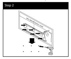
**1.** Match the TV BOTTOM LINE of WALL BRACKET INSTALL GUIDE with the bottom of TV and attach to the position.
