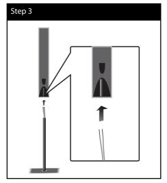
**4.** Attach the speaker to the pole, then secure the connection with a supplied screw.
