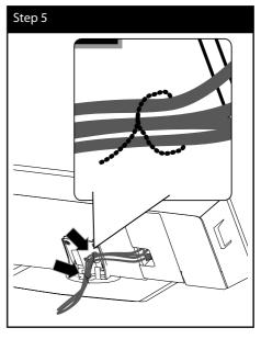
**6.** Assemble the rear cable cover as shown below.
