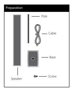
**1.** Attach the pole to the base, then secure the connection with a supplied screw.
