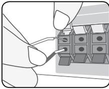
Connect the black end of each wire to the terminals marked -(minus) and the other end to the terminals marked + (plus).
