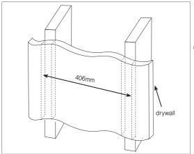
a. Locate and mark the centers of the wall studs using a stud finder.
