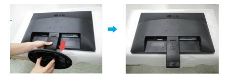
5. Pushing the PUSH button, Take the stand body from hinge body.
