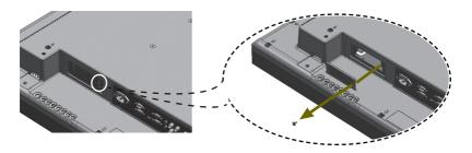
Attach the Box Guide to the rail slots, and press it upward.
