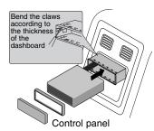
Before installing, make sure that the ignition-switch is set to OFF and remove the terminal of the car battery to avoid short-circuiting.
