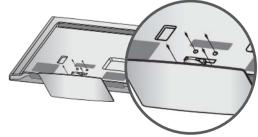
Assemble the parts of the Stand Rear Cover with the TV. (Only 32/42/47LD7\*\*\*, 32/37/42LD8\*\*\*)
