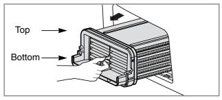
**4.** Clean the condenser completely under the tap letting water to flow through.
