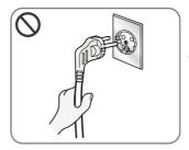
Disconnect the power cord by grasping the plug, not the cord.
