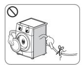
Before the appliance is removed from service or discarded, disassemble the door and cut off the power cord to prevent any future use.
