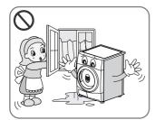
Do not install or store the dryer where it will be exposed to the weather.
