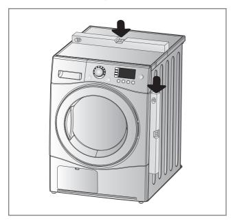
Leveling the dryer prevents undesirable noise and vibration. Place your dryer in solid and level Area.
