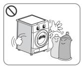
Do not dry articles that have been cleaned in, washed in, soaked in, or spotted with combustible or explosive substances (such as wax, oil, paint, gasoline, degreasers, dry-cleaning solvents, kerosene, etc.)
