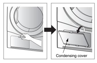
2. Open sealing cover by turning a locking lever.
