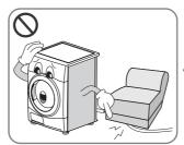
Do not kink, twist, crush or place heavy objects on power cord. Doing so may damage power cord.
