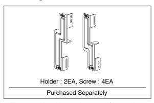
The stacking kit can be used for washer top plate size 550mm and 600mm for both.
