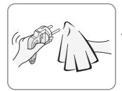
Wipe out the dirt and stains around the power cord and insert firmly into the socket
