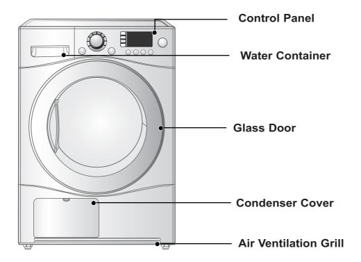
■ RC8011A1 / RC8011B1 / RC8011C1 / RC8011D1 / TD-C803E
