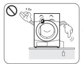
Before plugging power cord, make sure cord is earthed and connected to circuit breaker.
