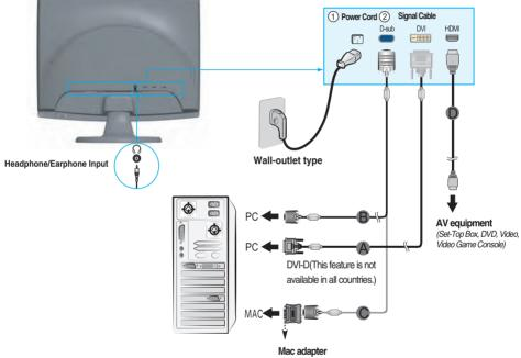
For Apple Macintosh use, a separate plug adapter is needed to change the 15 pin high density (3 row) D-sub VGA connector on the supplied cable to a 15 pin 2 row connector.
