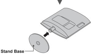
Use a **Coin** on the bottom of the stand base and turn the screw clockwise to tighten.
