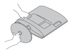
3 Turn the Stand Base Lock through 90° to separate the Stand Base from the Stand Body.
