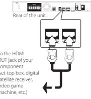
To the HDMI OUT jack of your component (set-top box, digital satellite receiver, video game machine, etc.)
