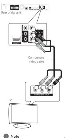
When you use COMPONENT VIDEO OUT connection, you can change the resolution for the output. (Refer to "Resolution setting" on page 23.)
