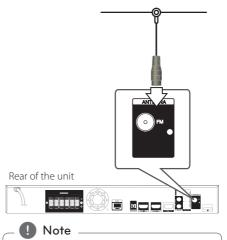
After connecting the FM wire antenna, keep it as horizontal as possible. Be sure to fully extend the FM wire antenna.
