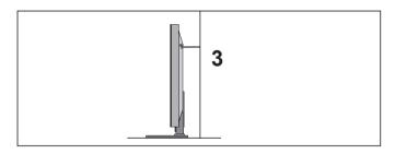
Use a sturdy rope to tie the product for alignment. It is safer to tie the rope so it becomes horizontal between the wall and the product.
