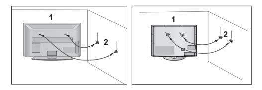
Use the eye-bolts or TV brackets/bolts to fix the product to the wall as shown in the picture. (If your TV has bolts in the eyebolts, loosen then bolts.)
