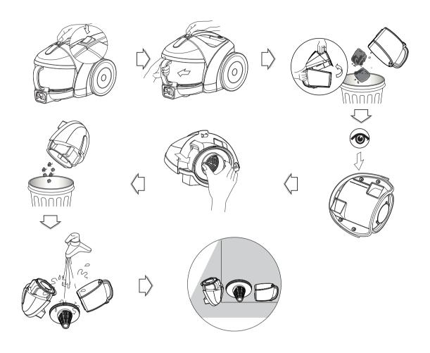
Push button and pull out dust tank. Raise dust tank cap.
