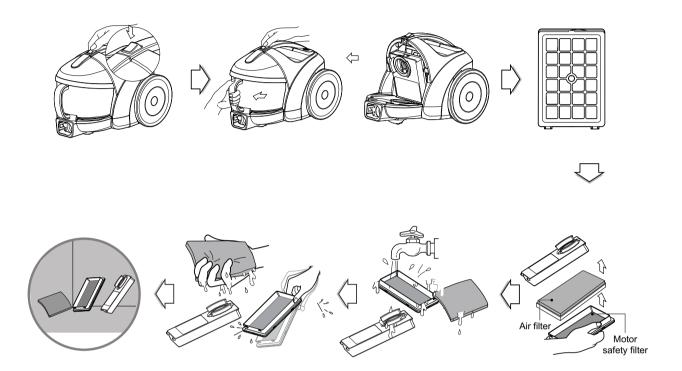
If suction power is decreased after cleaning dust tank, clean air filter and motor safety filter. Air filter and motor safety filter are located at the center of vacuum cleaner in the above figure.
