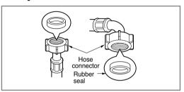
Two rubber seals are supplied with the water inlet hoses.
