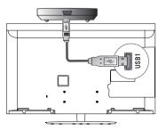
3 Attach the RF Dongle to the velcro as shown below and then turn on the TV.
