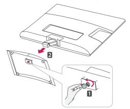
3 Remove 2 screws and pull out the **Stand Body** from the Monitor set.
