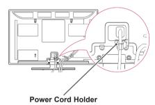
2 Gather and bind the cables with the Cable Holder. Install the LAN cable as shown to reduce the electromagnetic wave.
