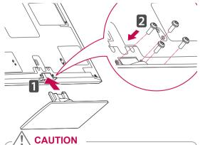
Tighten the screws firmly to prevent the TV from tilting forward. Do not over tighten. Only 50/60PZ75\*\*, 50/60PZ95\*\*
