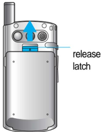
To remove the battery from the phone, push the battery release latch and then pull out the battery from the phone.
