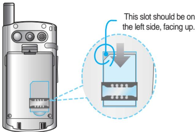
To insert the card into the phone, push the card into the metal strip until it clicks and locks into place.
