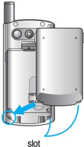
To install the battery into the phone, insert the battery into the battery slot at a slight angle and press the top of the battery until the battery clicks and locks into place.
