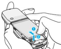
1. Position the lugs on the top of the battery into the retaining holder.
