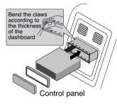
Before installing, make sure that the ignition-switch is set to OFF and remove the terminal of the car battery to avoid short-circuiting.
