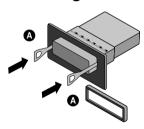
If there is already an installation sleeve for the receiver unit in the dashboard, it must be removed.
