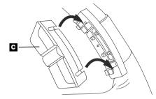
4. When removing the remote control unit from the holder, move the corrugated release section toward the steering wheel as far as possible before sliding the remote control unit toward you.
