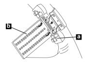
2. Cut the extra portion of the belt at the center of the cover holder.
