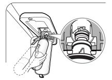
Rotate the water filter up into position and close the cover. The cover will click when closed correctly.
