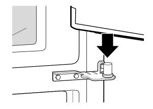
1 Lower the door onto the middle hinge pin. Make sure that the plastic sleeve is inserted into the bottom of the door.
