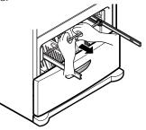
2 Grasp the drawer on each side and hook the door supports (1) into the rail tabs (2) located on both sides.
