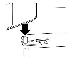
1 Lower the door onto the middle hinge pin.
