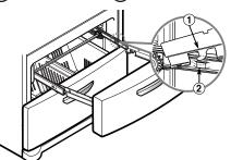
3 Lower the door into final position and tighten the screws located on both sides.
