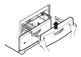
4 With both hands, flex the center bar enough to allow the gears on both ends to release from the track.
