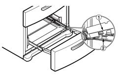
3 Lower the door into final position and tighten the screws (3) located on both sides.
