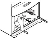
2 Grasp the drawer on each side and hook the door supports (1) into the rail tabs (2) located on both sides.
