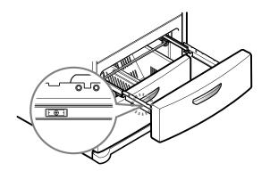
3 Grasp the drawer on each side and pull it up to separate it from the rails.
