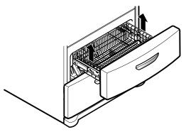
2 Remove the screws on both the left and right rails.
