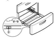
4 With the drawer pulled out to full extension, insert the basket in the rail assembly.
