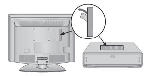
Attach the set-top box to the TV by pressing the Velcro strips together.
