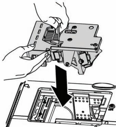
**Note:** The lamp module must sit securely in place and the lamp connector must be connected properly before tightening the screws.
