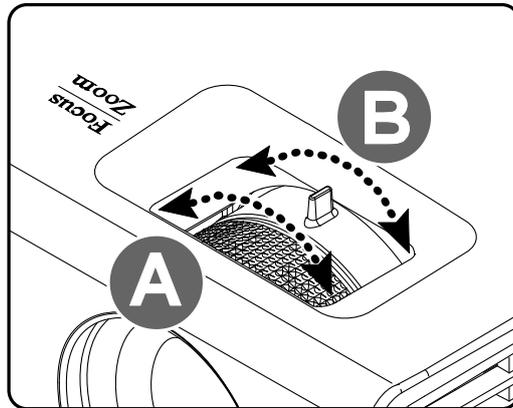
2. Use the **Image-focus** control (on the projector only) to sharpen the projected image **A**.
