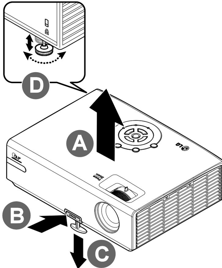
1. To raise the level of the projector, lift the projector [A] and press the height-adjuster button [B].
