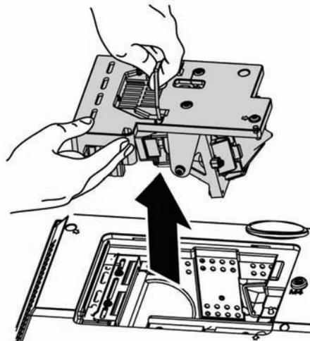
6. Reverse steps 1 to 5 to install the new lamp module. While installing, align the lamp module with the connector and ensure it is level to avoid damage.
