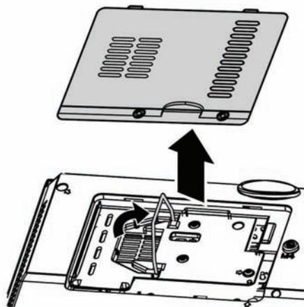
3. Remove the two screws from the lamp module.
