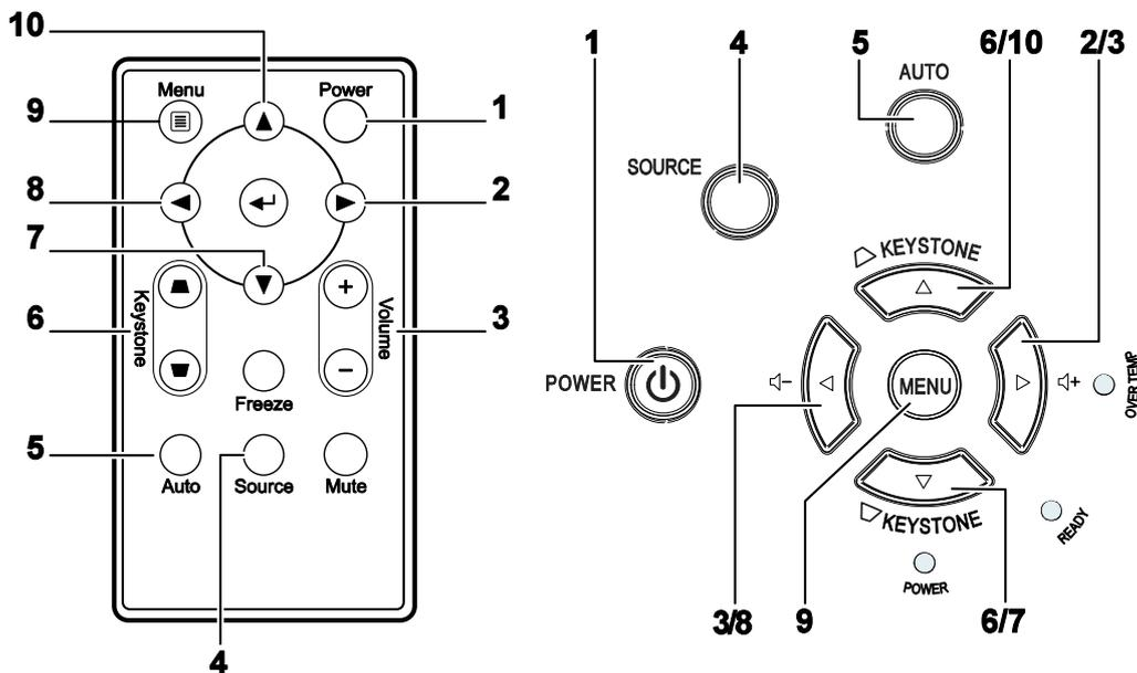
Some buttons on the projector have multiple functions. For example, item 6/7 on the projector functions as the keystone button and as the down cursor key.
