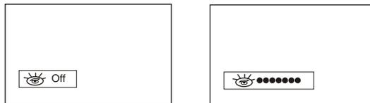
When the eye function is **On** the most suitable picture is automatically adjusted according to the surrounding conditions.
