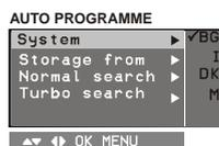
4. If this station is the one required, press the ▲/▼ button to select **Storage**. Select the desired programme number (0 to 199) with the ◀/▶ button or NUMBER buttons. Any number under 10 is entered with a numeric '0' (or '00') in front of it, i.e. '05' (or '005') for 5.
