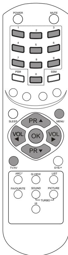
Up to 200 TV stations can be stored in this set by programme numbers (0 to 199). Once you have preset the stations, you will be able to use the ▲/▼ or NUMBER buttons to scan the stations you programmed. Stations can be tuned using automatic or manual modes.
