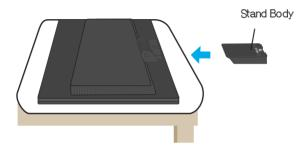
**3.** Assemble the Stand Base(Front, Rear) into the Stand Body in the correct direction.
