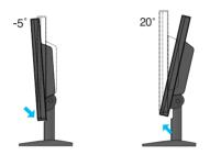
Warning: When adjusting the angle of the screen, do not put your finger(s) in between the head of the monitor and the stand body . You can hurt your finger(s).
