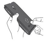
2 Slide the SIM card into the SIM card holder. Make sure the gold contact area on the card is facing downwards.
